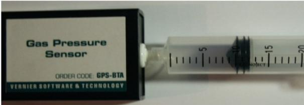
A black rectangular sensor labeled 'Gas Pressure Sensor' with 'ORDER CODE: GPS-BTA' and 'VERNIER SOFTWARE & TECHNOLOGY' is connected to a clear plastic syringe with a black plunger.
